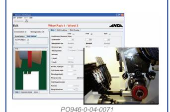
This software enables the automatic white-sticking option within the dresser software. This allows automatic sticking of super-abrasive grinding wheels.
