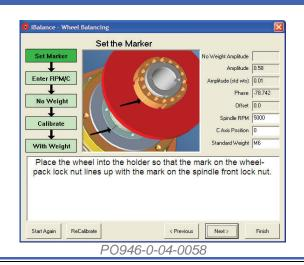
Balanced wheel packs is important to achieve superior surface finish and wheel life. iBalance will semi-automatically balance the wheel pack inside the machine using a software assistant.
