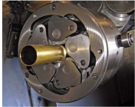
Rolling on pipes with WAGNER® RS 60-5
