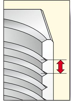
For internal threads, as a general rule, when the ratio between cutting tool dia. ( $D_2$ ) and the thread dia. (minor dia.) is below 70% the profile distortion is neglected.
