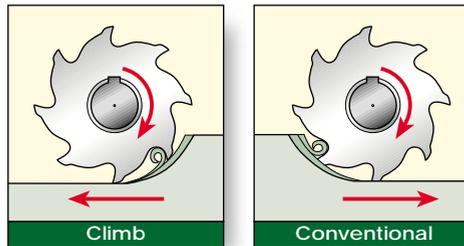
In conventional milling, friction and rubbing occur as the insert enters into the cut, resulting in chip welding and heat dissipation into the insert and workpiece.
